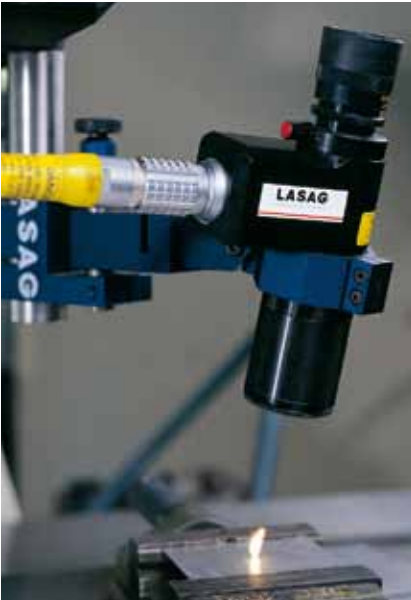
Welding with Fiber Optic Processing head
