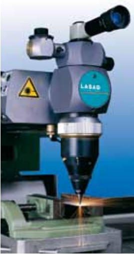
Cutting with BAK 4
