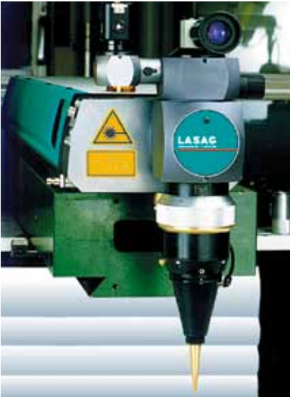
Drilling with the BAK4 head
